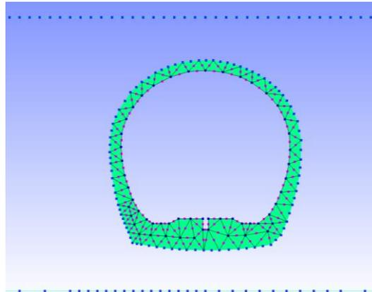
*Example of a hybrid mesh: FEM mesh for the tunnel structure and BEM mesh for ground layers*
